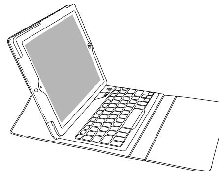
2 Press the On/Off Switch for 1.5 to 5 seconds. The Power Indicator Light
