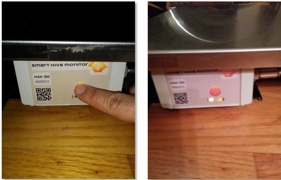
4. Place the beehive centered on top of the SHM. Make sure the ON/OFF switch remains in the ON position.
