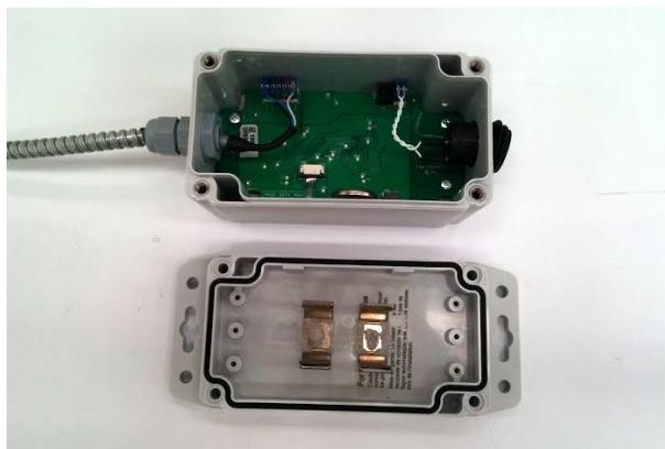
5. If you are **replacing** a battery, there will already be a battery in the module. In this case, the battery is connected to the printed circuit board with a lock connector. Pinch/press the connector to pull the male connector loose from the female connector on the printed circuit board. This operation may take some wiggling of the connector to remove it.
