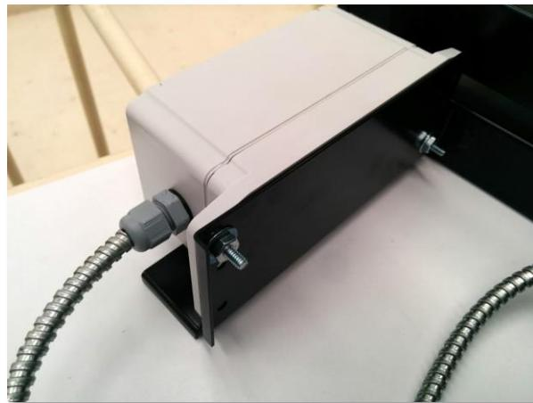
13. Reattach the top cover. You are done. Turn the power switch to the on – “I” position. Try to communicate with the module with a smartphone as per the Installation Guide.
