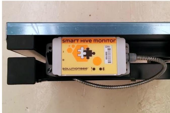
2. Remove the top plate. Identify the two screws (and washers and nuts) that attach the electronic module to the frame bracket.
