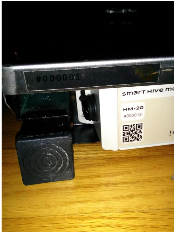
3. Zeroing the scale: Without the hive on top of the monitor, zero out the scale by pressing the orange button for between 5 and 20 seconds. The yellow warning light will blink for two seconds indicating that zeroing was successful.
