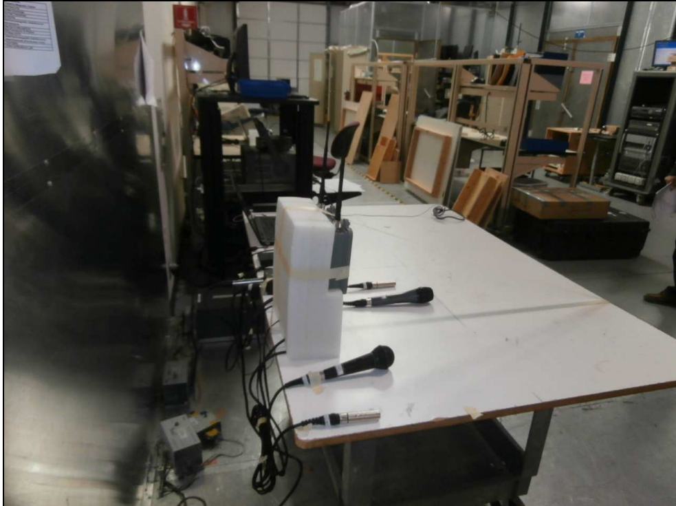
Figure 8: Test Setup Photo – Conducted Emissions – Breakout Box Computer Configuration
