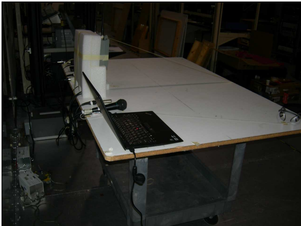
Figure 6: Test Setup Photo – Conducted Emissions – Breakout Box Configuration
