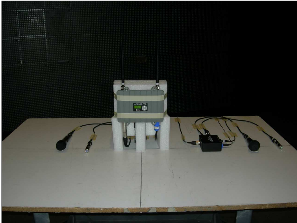
Figure 1: Test Setup Photo – Radiated Emissions
