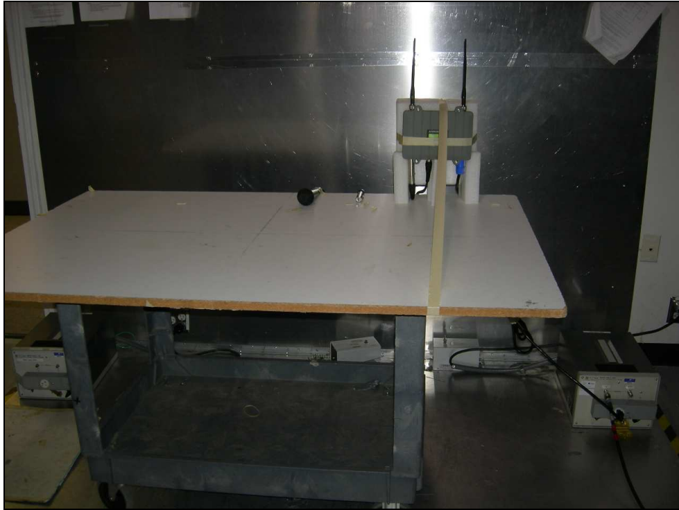
Figure 3: Test Setup Photo – Conducted Emissions – AiRocks Configuration
