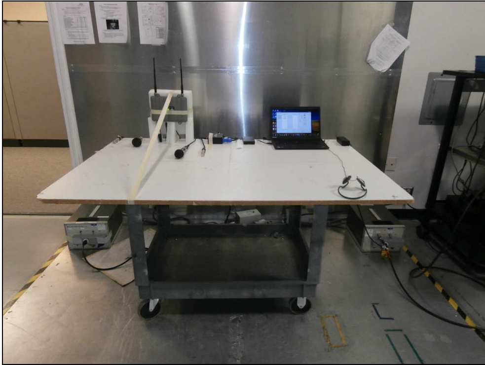
Figure 7: Test Setup Photo – Conducted Emissions – Breakout Box Computer Configuration
