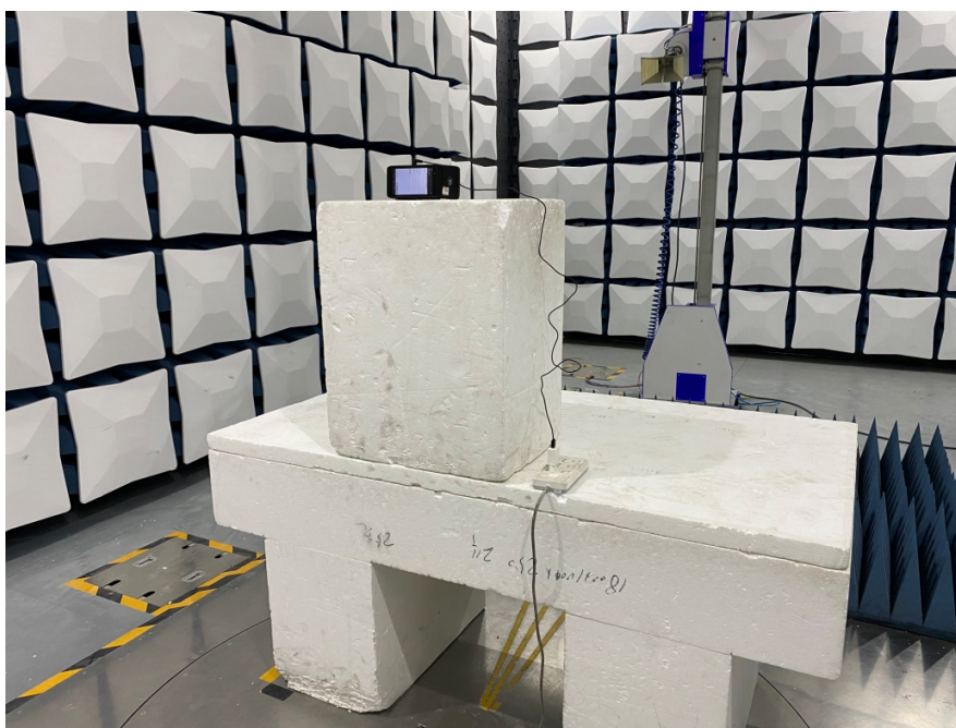
Radiated Emissions View (1GHz-18GHz)
