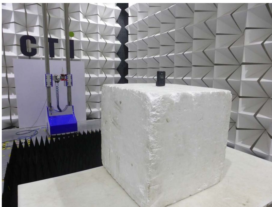
Radiated spurious emission Test Setup-2(Above 1GHz)
