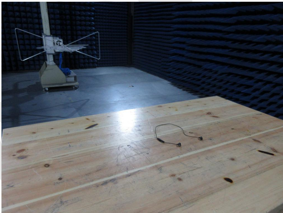
Photo of Radiation Emission Test
