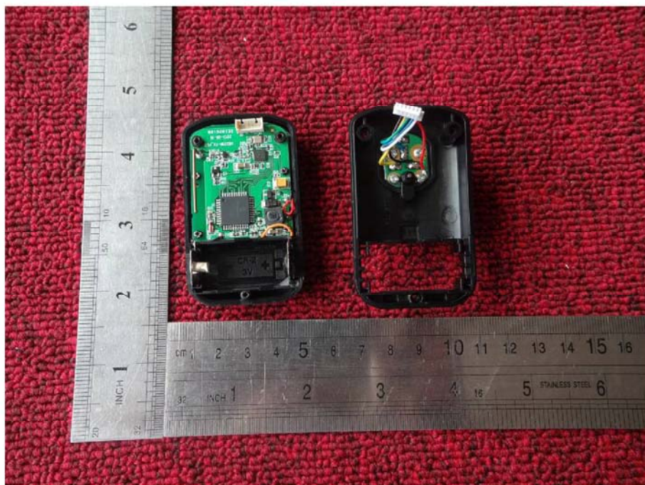
Internal photograph of EUT-Transmitter
