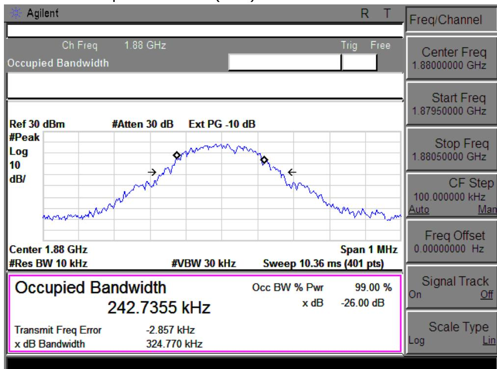
Occupied Bandwidth (99%) GPRS 1900 BAND CH 810
