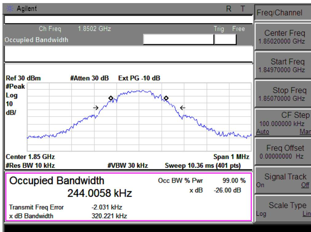
Occupied Bandwidth (99%) GPRS 1900 BAND CH 661
