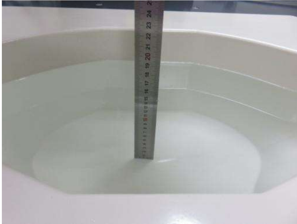
Photograph of the depth in the Body Phantom (835MHz, 16.1cm depth)
