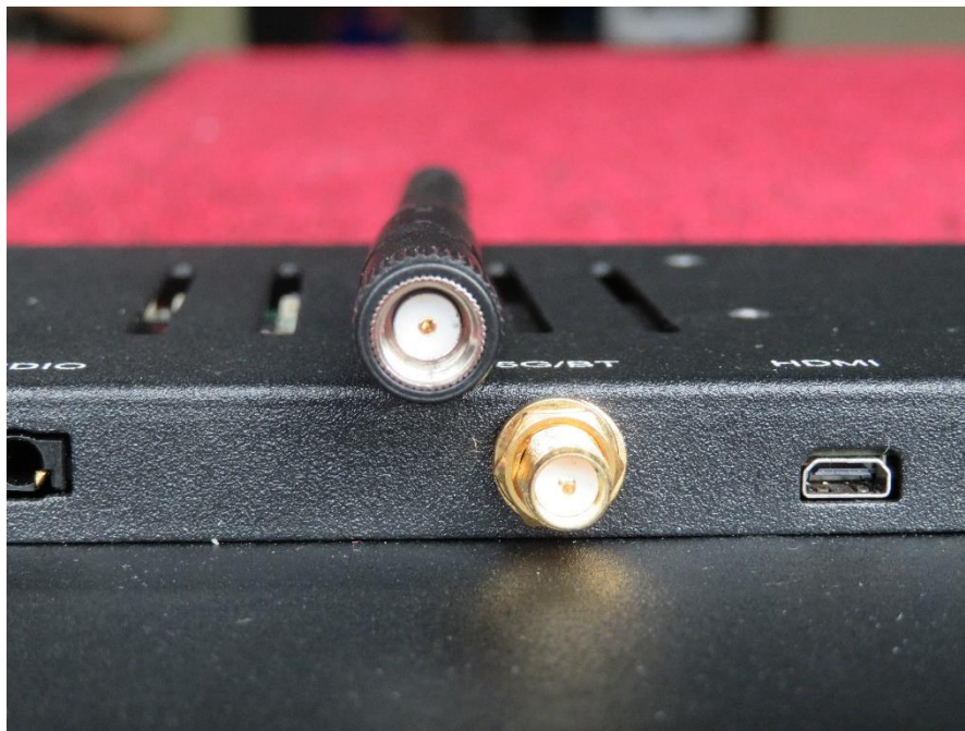
PR-SMA antenna detail photograph
