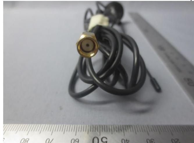
A photograph showing a coiled black cable with a gold-colored reverse-SMA connector. The cable is positioned next to a metric ruler. |
