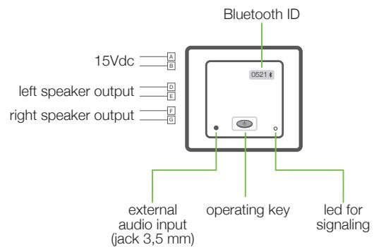
**External audio input:** the Module includes an external audio input (3,5mm jack). When the user inserts a jack the audio output switches to the signal from the external audio source (red led) and overrides the Bluetooth mode.
