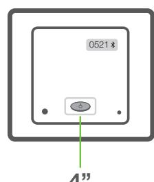
**3.2.** Once the blue led flashes you are ready to pair. The Module remains in pairing mode for one minute. If the Bluetooth device is not connected during this time, the Module will automatically turn off and you must repeat the process again.
