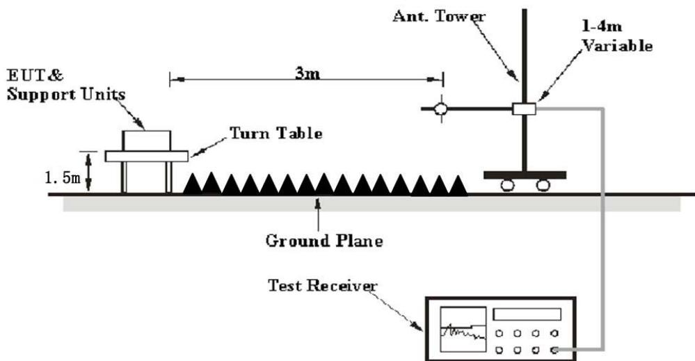
The radiated emission and out of band emission tests were performed in the 3 meters chamber test site, using the setup accordance with the ANSI C63.10-2013. The specification used was the FCC part 15.209, 15.205 and FCC part 15.249 limits.
