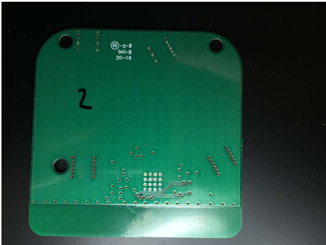
Figure 3 - SwipeSense Badge PWB back side
