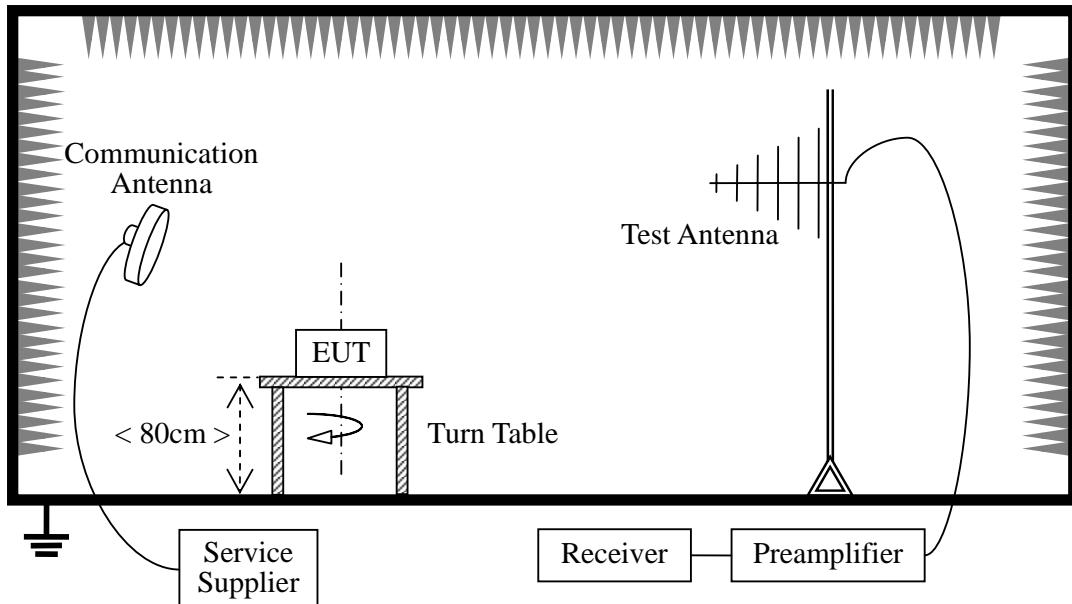
The EUT is powered by the Battery charged with the AC Adapter which is powered by 120V, 60Hz AC mains supply. The Module is located in a 3m Semi-Anechoic Chamber; the antenna factors, cable loss and so on of the site as factors are calculated to correct the reading. During the measurement, the EUT is activated and transmitting with the other Bluetooth device (Supply by the Applicant) during the test.
