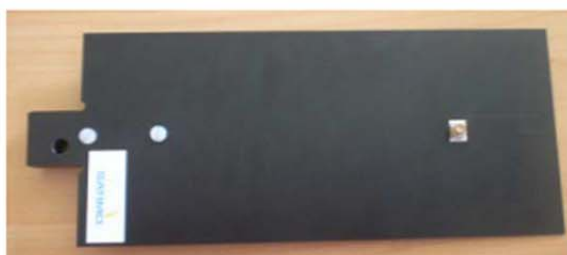
Figure 1 – Satimo COMOHAC Validation Dipole
