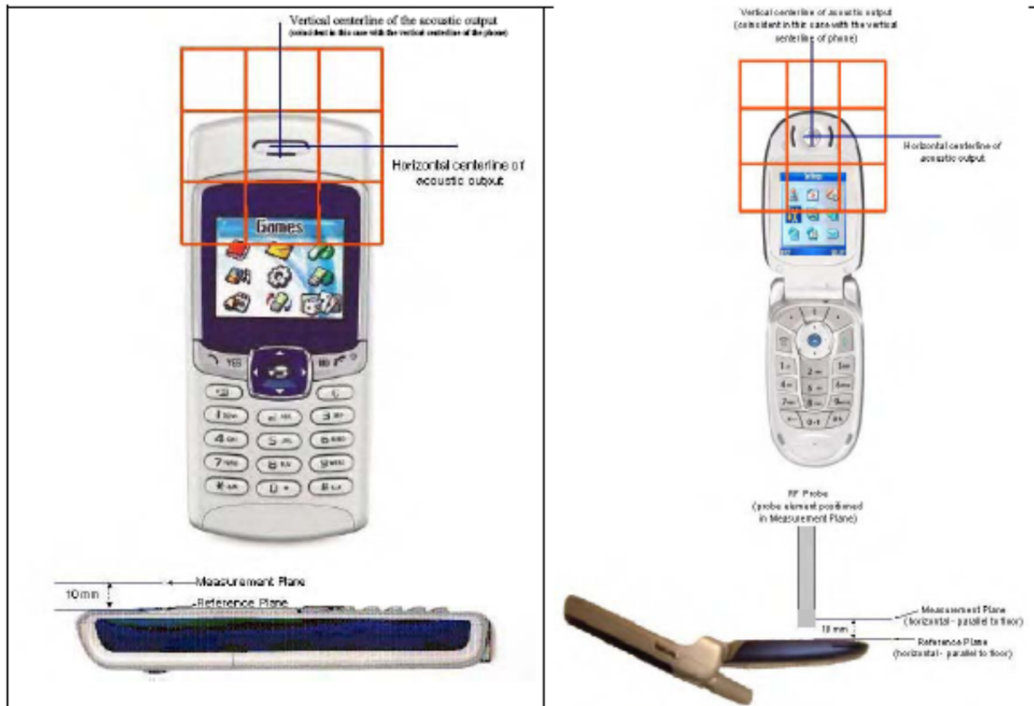
Reference and plane for RF emission measurements
