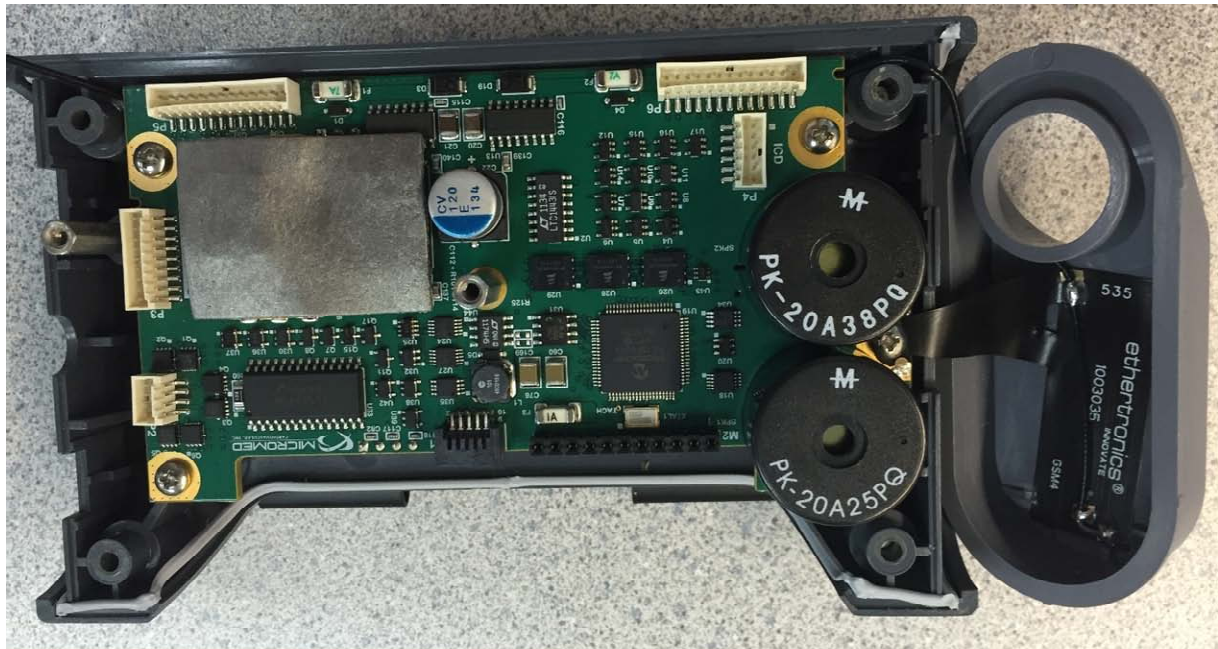
Antenna (M10418) Position within Right Housing (M10076)
