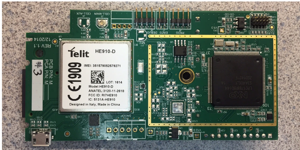
Remote Monitoring Module Board (M10419) (Bottom)
