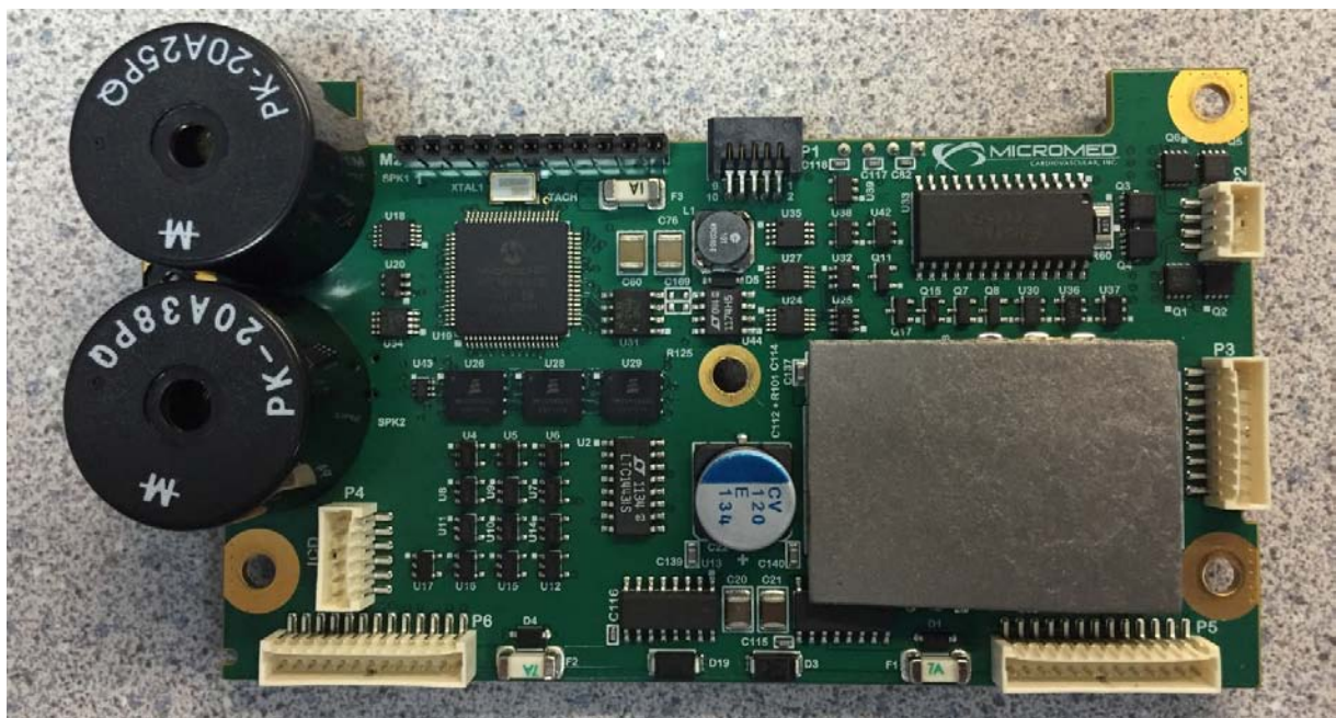
Main Board (M10277) with RF Absorber material (M10378) (Top)
