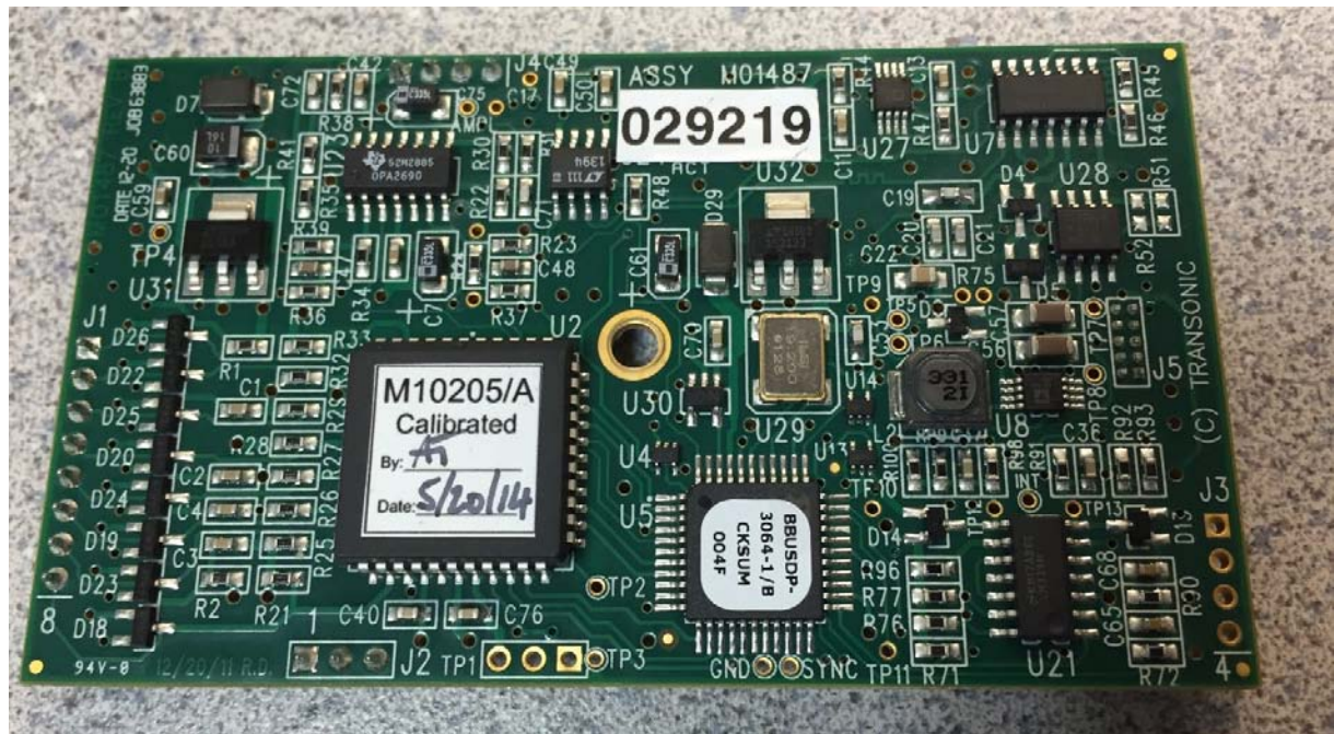
Flow Meter Board (M10205) with RF Absorber Material (M10376 & M10377) (Bottom)
