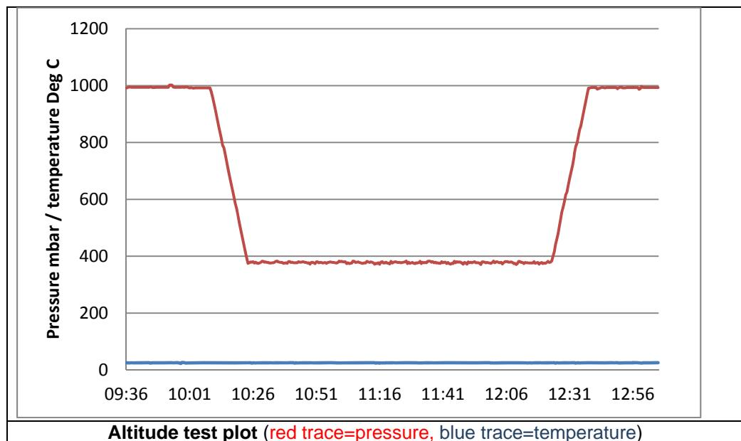
Note – A correction error of -7 mbar needs to be applied to the above plot to ascertain a more accurate reading.
