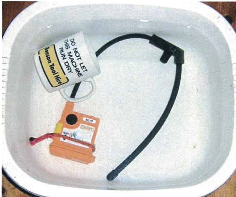
Figure A.1 – Thermal shock submersion in water
