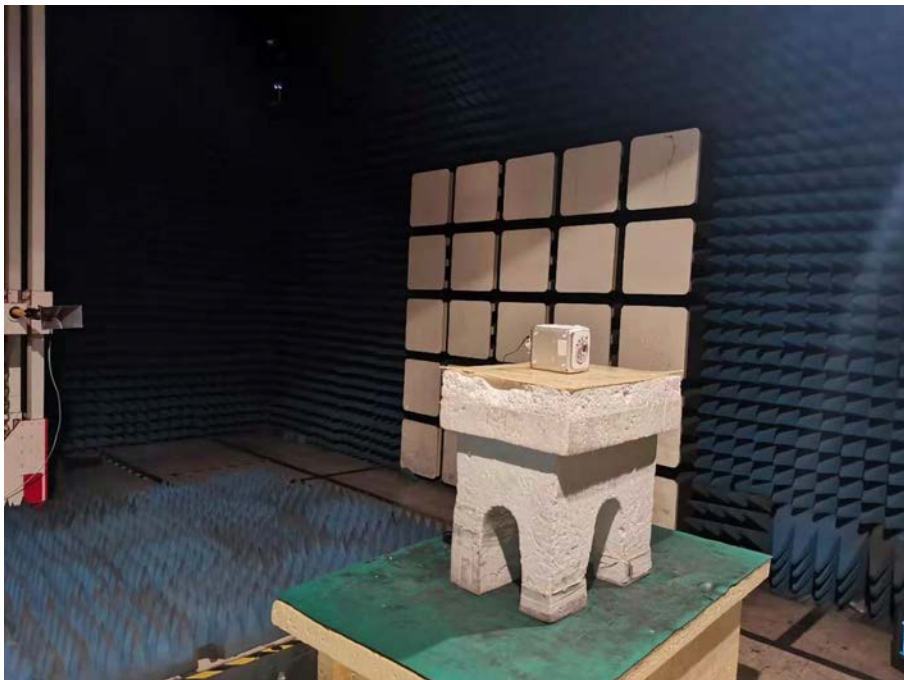
Spurious Emission Test Setup (Above 1GHz)
