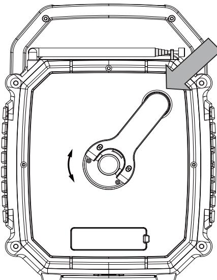
2. Continue turning the Crank to generate electricity to charge the internal battery. More power is generated the longer you turn the crank handle, and the Radio listening time will be extended (Radio reception only).
