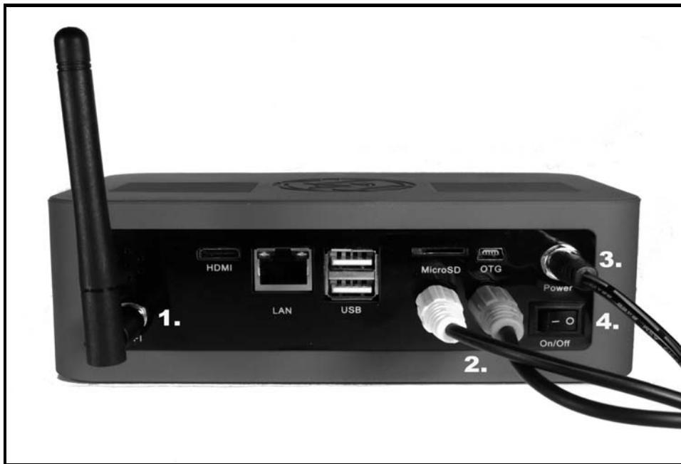
1. CONNECT THE WI-FI ANTENNA by holding the threaded end and screwing it clockwise onto the “WIFI” connector on the back of the player. Bend the antenna 90° at its hinged joint, and rotate the antenna (if necessary) so that the tip is pointing straight up.
