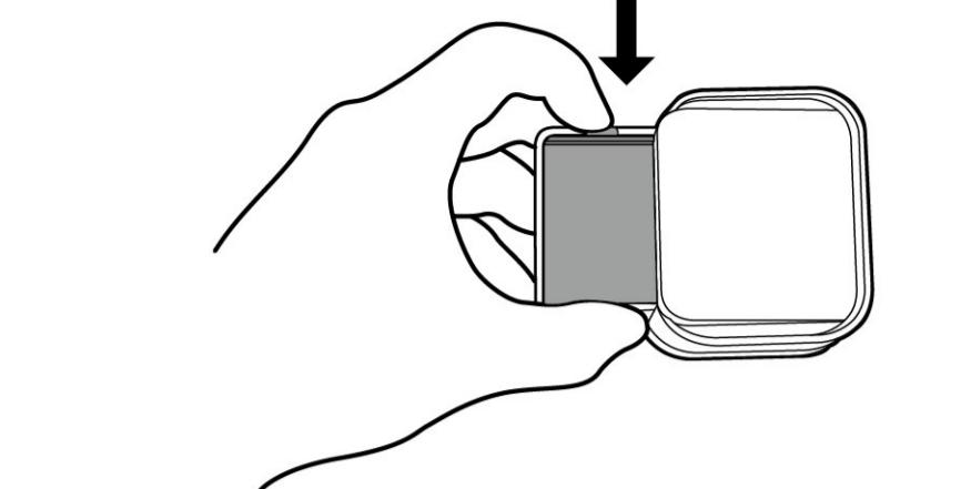
Remove the door. Slide the end of the charging cable into the opening and press the cable down into the slots.
