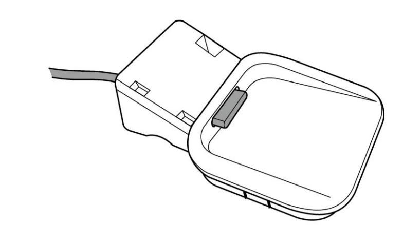
Place the adapter in the base station by pressing it down and back into position.
