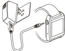
Please connect the accessory cable to the USB interface on the computer or a 5V DC charger. Insert the headphone plug into the headphone jack and start charging. After 2-3 hours, the battery will be full. Then, unplug the cable.
