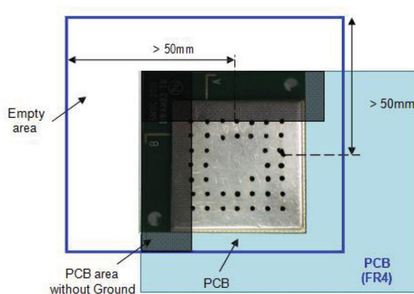
**Typical Module (RF) Placement:** >30mm separation (all directions) from antennae is recommended.
