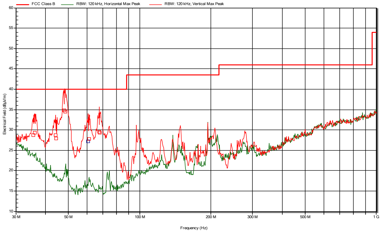
Figure 8: Electric field emissions Plot, 30MHz to 1GHz
