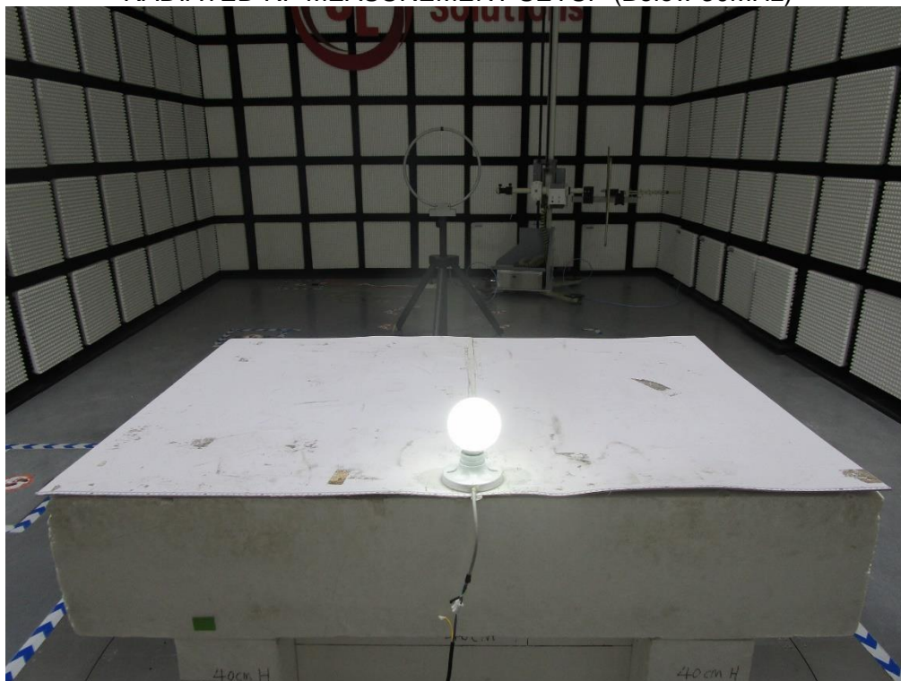
RADIATED RF MEASUREMENT SETUP (Below 30MHz)
