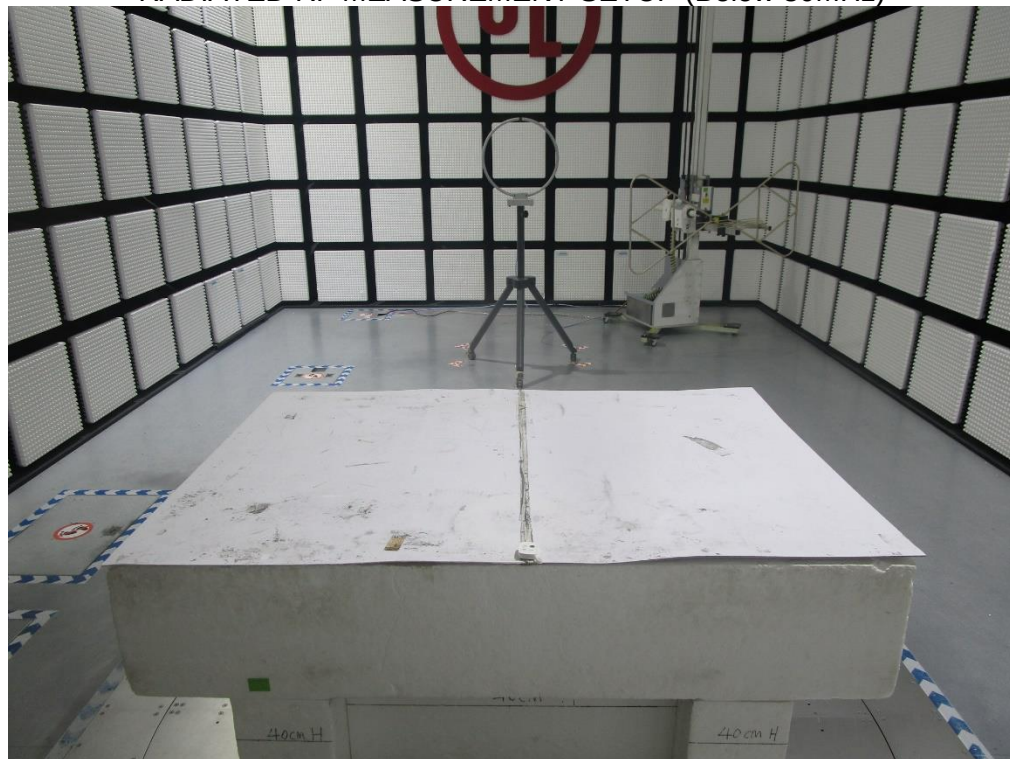
RADIATED RF MEASUREMENT SETUP (Below 30MHz)
