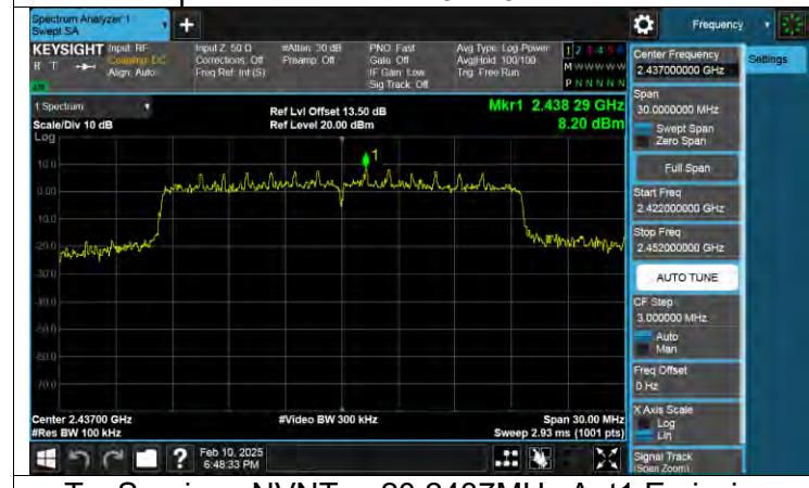
**Tx. Spurious NVNT ax20 2437MHz Ant1 Emission**
