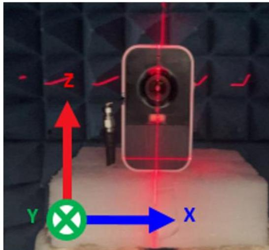
A photograph of an antenna setup. A black rectangular device with a circular lens is mounted on a white rectangular base. Red laser beams are emitted from the top and bottom of the device. A coordinate system is overlaid on the image, showing a red arrow pointing upwards (Y-axis), a blue arrow pointing to the right (X-axis), and a green circle with a crosshair at the origin. |
