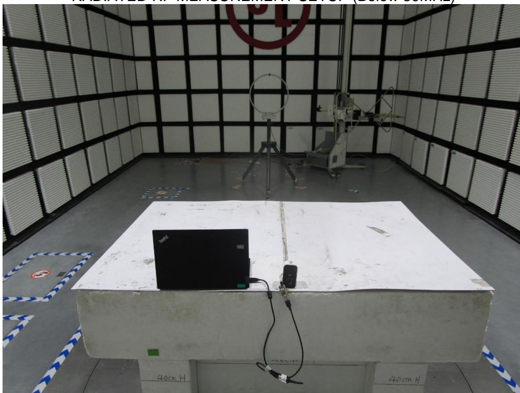
RADIATED RF MEASUREMENT SETUP (Below 30MHz)
