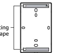
2. Remove backing on the other side of the mounting tape and carefully push the wall plate onto your mounting surface.
