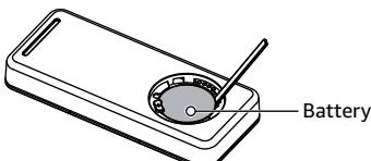
3. Push the battery cover back onto the smart remote.
