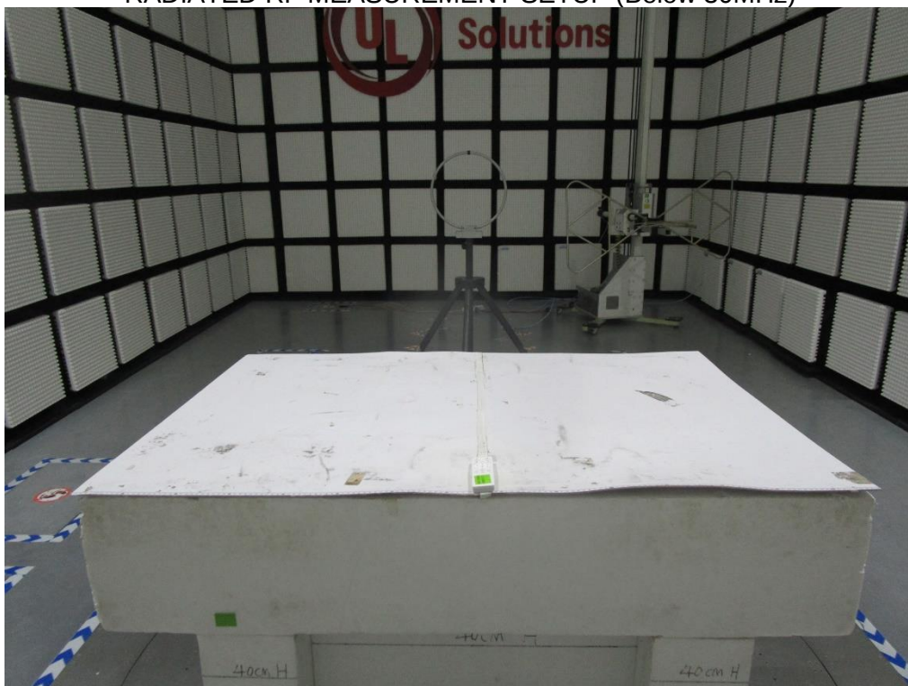
RADIATED RF MEASUREMENT SETUP (Below 30MHz)
