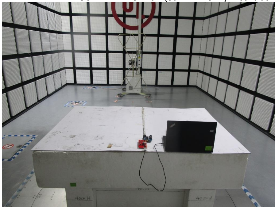
RADIATED RF MEASUREMENT SETUP (30MHz~1GHz) ---condition 1
