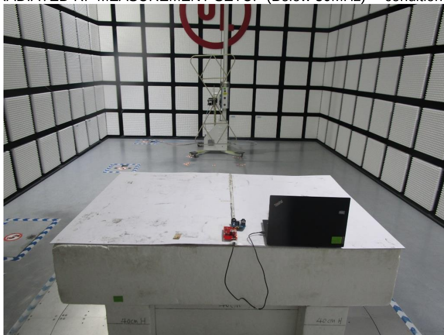
RADIATED RF MEASUREMENT SETUP (Below 30MHz) ---condition 1
