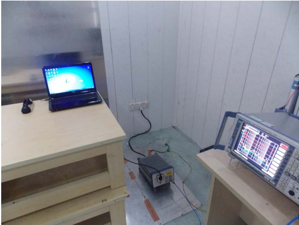
FCC RADIATED EMISSION TEST SETUP
