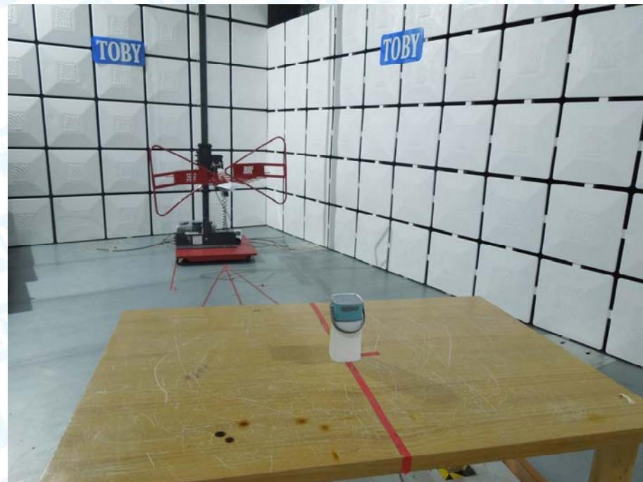
**Photo of Setup for Conducted Emission**
