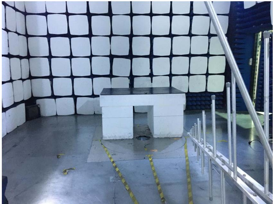
Radiation Emission Test Setup (30MHz to 1GHz)
