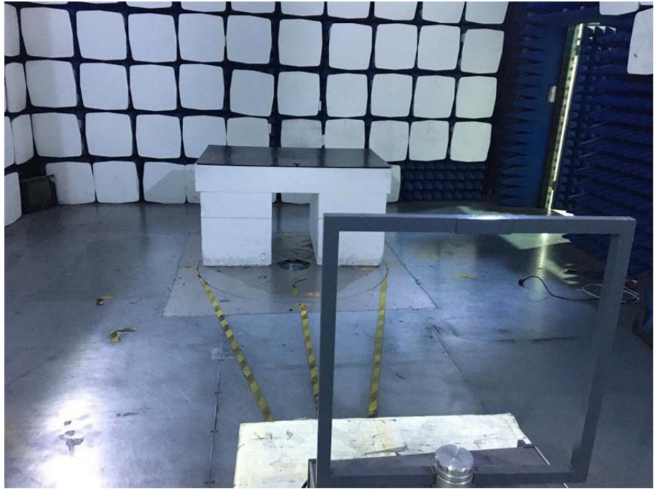
Radiation Emission Test Setup (Below 30MHz)
