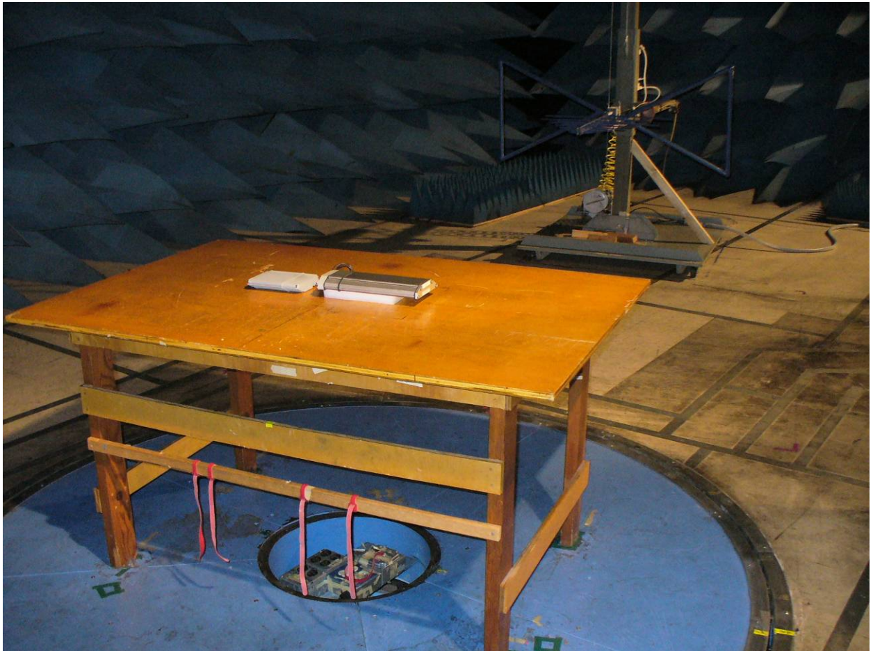
Figure 5: Radiated Emissions Test Setup – Internal Antenna - Rear View 1 – EUT Flat
