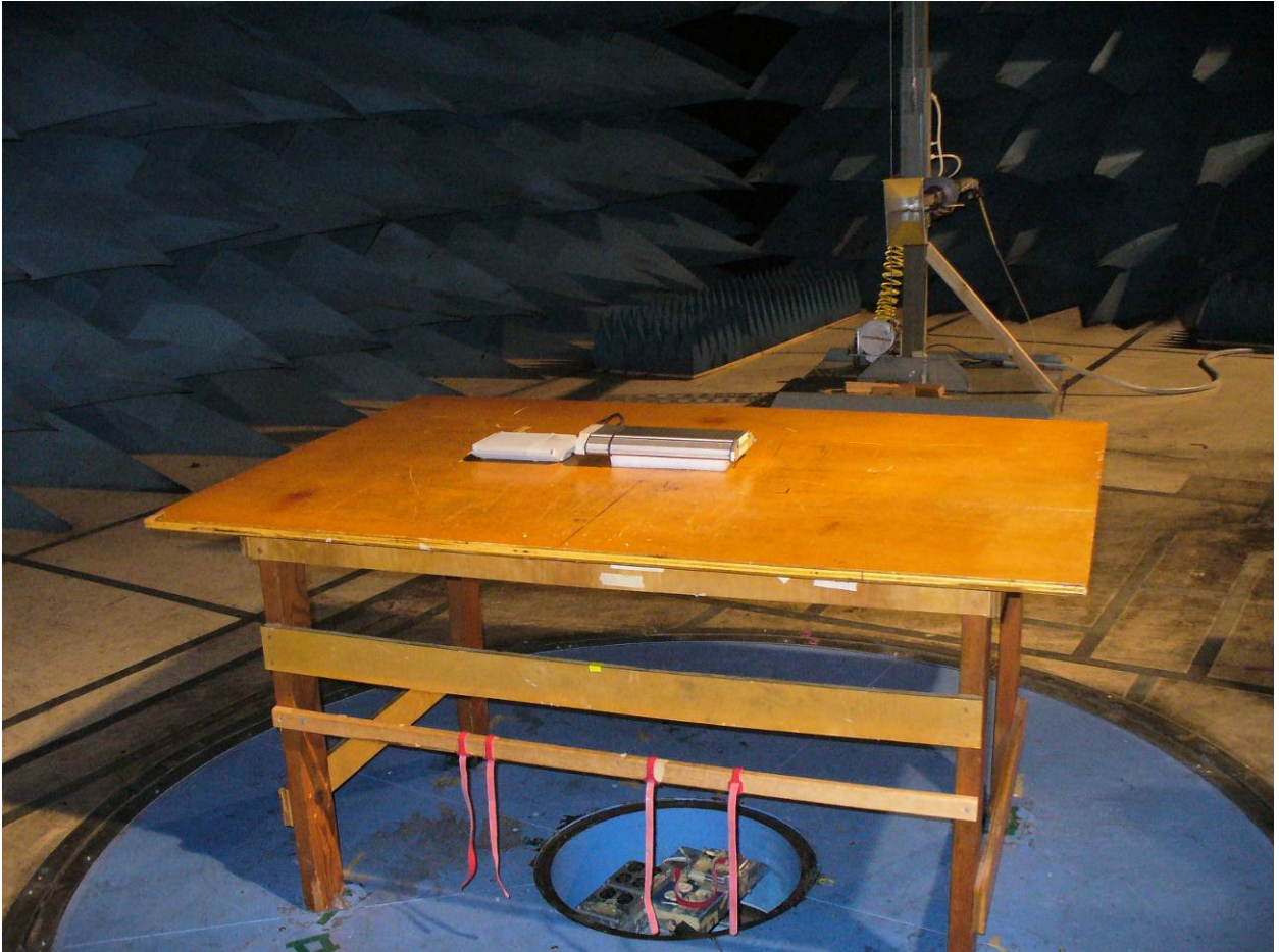
Figure 6: Radiated Emissions Test Setup – Internal Antenna -Rear View 2 – EUT Flat
