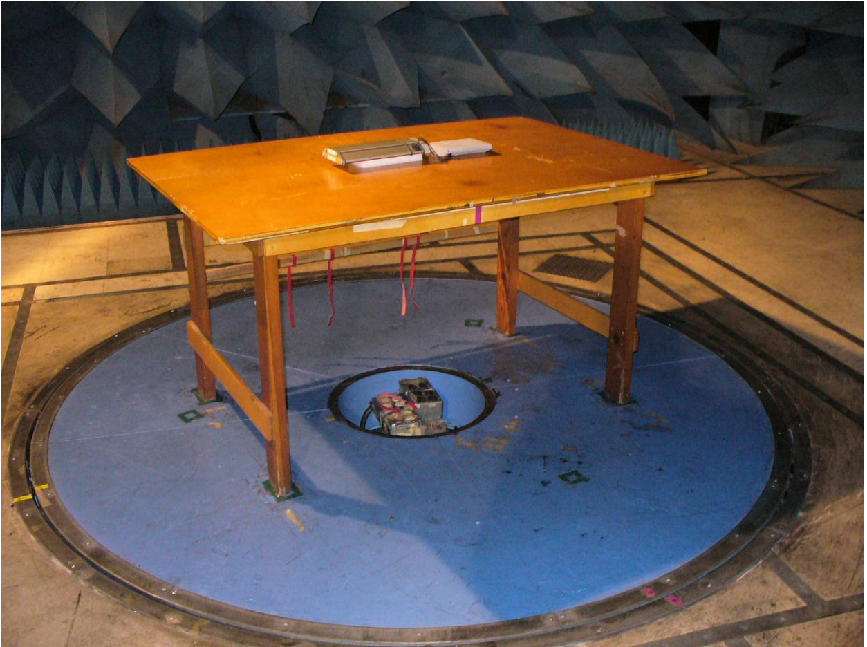
Figure 4: Radiated Emissions Test Setup – Internal Antenna - Front View – EUT Flat
