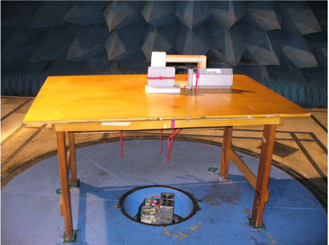
Figure 1: Radiated Emissions Test Setup – External Antenna - Front View – EUT on Side
