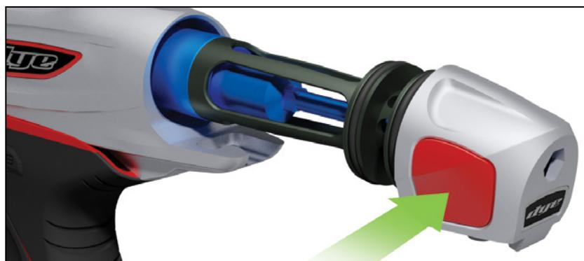
To remove the bolt, grab the bolt back cap with your right hand. Push the bolt release button, located on the left side of the bolt back cap, with your thumb. With the bolt release button depressed pull firmly back on the bolt.
