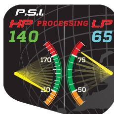
The screen will read "Processing" and display HP and LP psi. When done, press the center of the joystick, and continue to scroll through the Data Settings menu.
