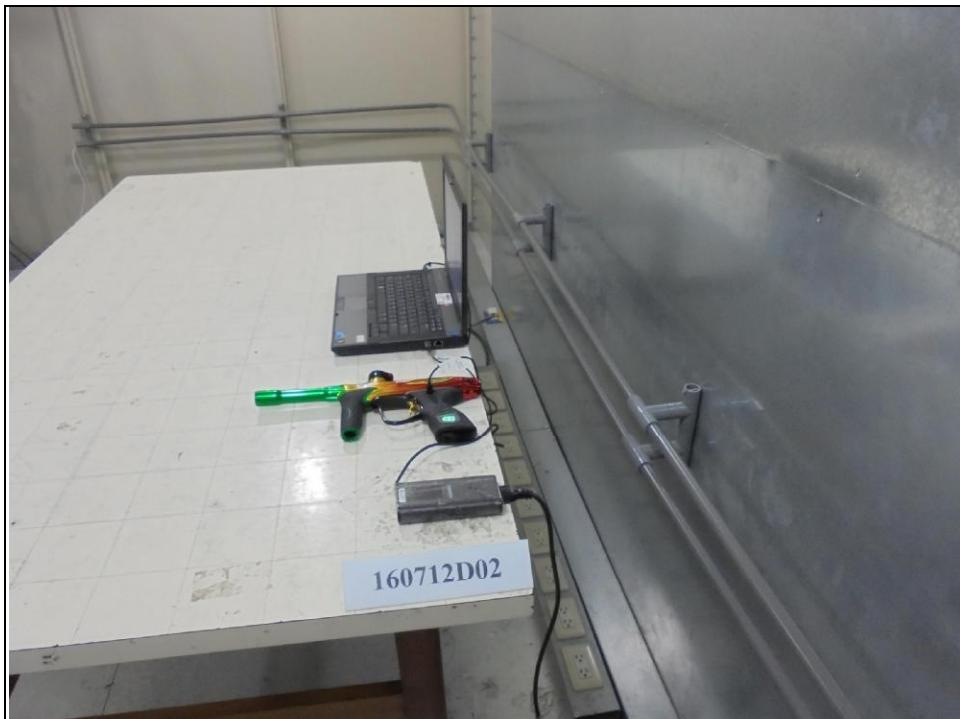
RADIATED EMISSION TEST - Mode A
