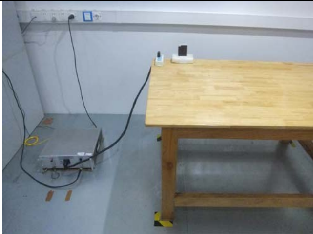
Conducted Emissions Test Setup Front View
