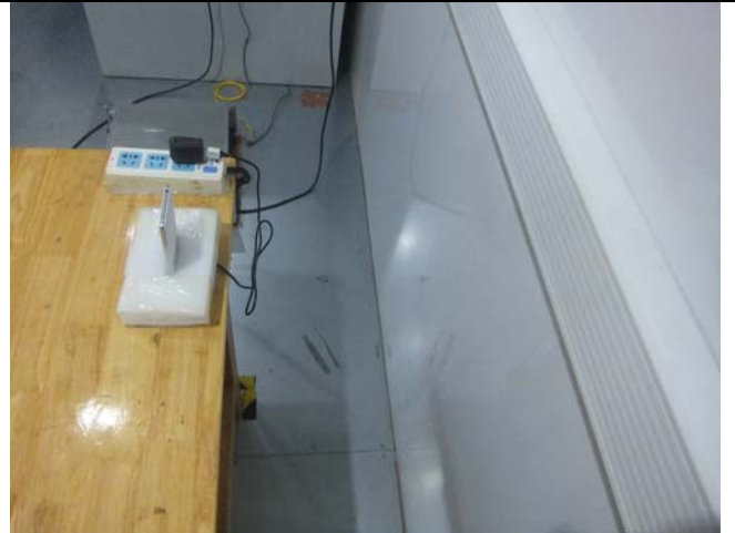
Conducted Emissions Test Setup Side View
