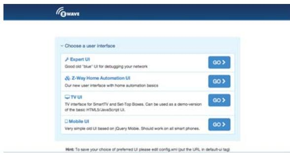
When going to <http://YOURIP:8083> you will see a selection menu to choose the web based UI you like to work with. The two most interesting UIs are the **Z-Wave Expert UI** (to create and manage the Z-Wave Network) and the **Z-Way Home Automation** user interface for day-by-day usage of the whole system. Above and beyond this you can use various mobile platform native apps you find in the app stores to access the system.
