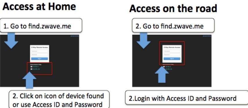
Whenever you access [find.zwave.me](http://find.zwave.me) again and a local RaZberry is found clicking on the IP address will lead you right to your Smart Home User Interface. If your Pi uses a fixed IP address this address can be used for direct IP access without using the [find.zwave.me](http://find.zwave.me) service. You can even turn off
