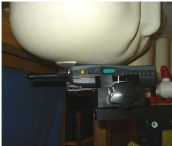
Held-to-Ear Test Setup – FT4 S_1c ig, Antenna 1, Right ear touch position
