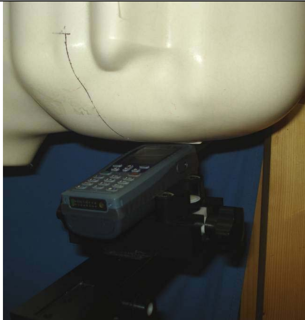
Held-to-Ear Test Setup – FT4 S_1c ig, Antenna 1, Left ear tilt position
