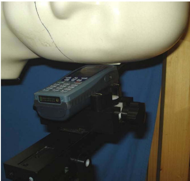
Held-to-Ear Test Setup – FT4 S_1c ig, Antenna 2, Left ear tilt position
