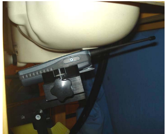
Held-to-Ear Test Setup – FT4 S_1c ig, Antenna 2, Left ear tilt position
