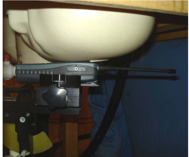
Held-to-Ear Test Setup – FT4 S_1c ig, Antenna 2, Left ear touch position
