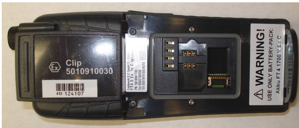
Back of FT4 S Ex_1c C ig (Intrinsically Safe variant) without battery
