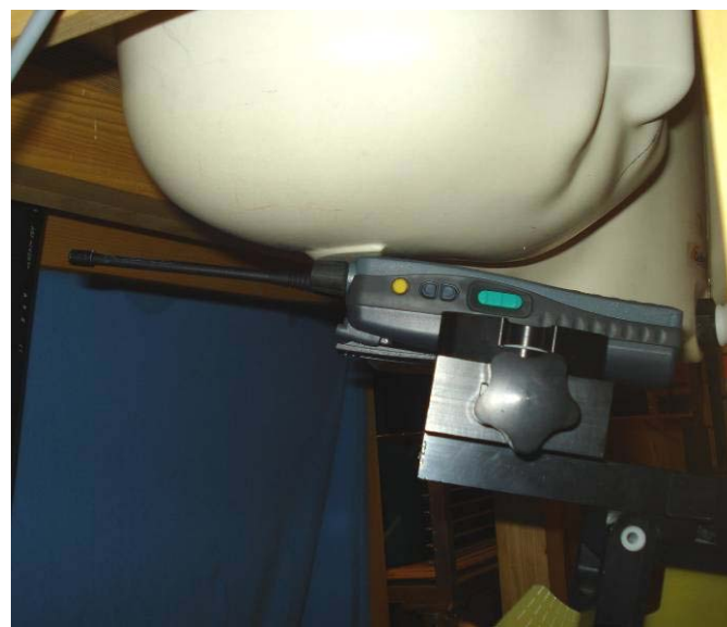
Held-to-Ear Test Setup – FT4 S_1c ig, Antenna 2, Right ear tilt position
