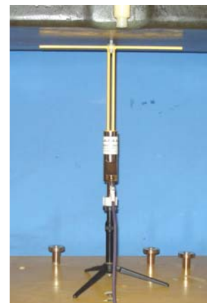
SPEAG 450 MHz Validation Dipole Setup
