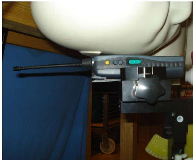
Held-to-Ear Test Setup – FT4 S_1c ig, Antenna 2, Right ear touch position
