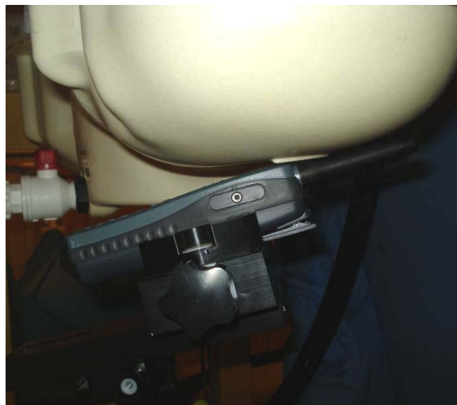
Held-to-Ear Test Setup – FT4 S_1c ig, Antenna 1, Left ear tilt position
