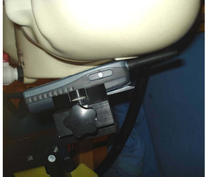
Held-to-Ear Test Setup – FT4 S Ex_1c C ig, Antenna 1, Left ear tilt position
