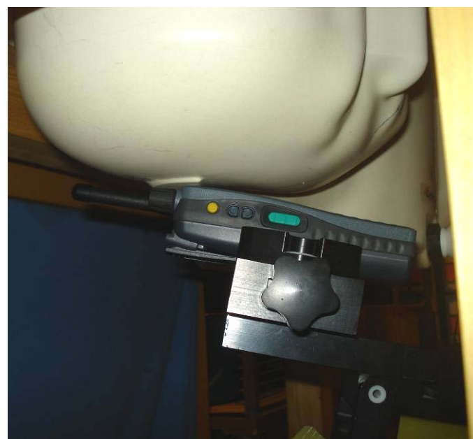
Held-to-Ear Test Setup – FT4 S_1c ig, Antenna 1, Right ear tilt position
