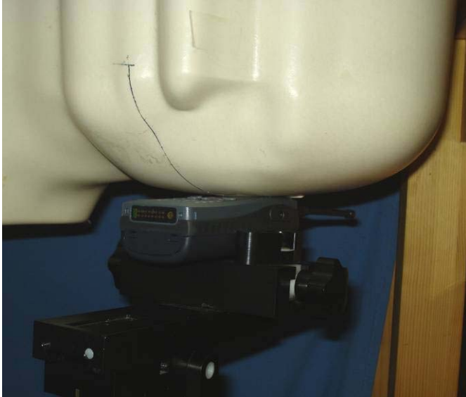
Held-to-Ear Test Setup – FT4 S_1c ig, Antenna 2, Left ear touch position
