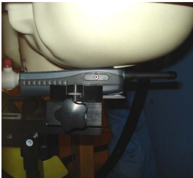
Held-to-Ear Test Setup – FT4 S_1c ig, Antenna 1, Left ear touch position
