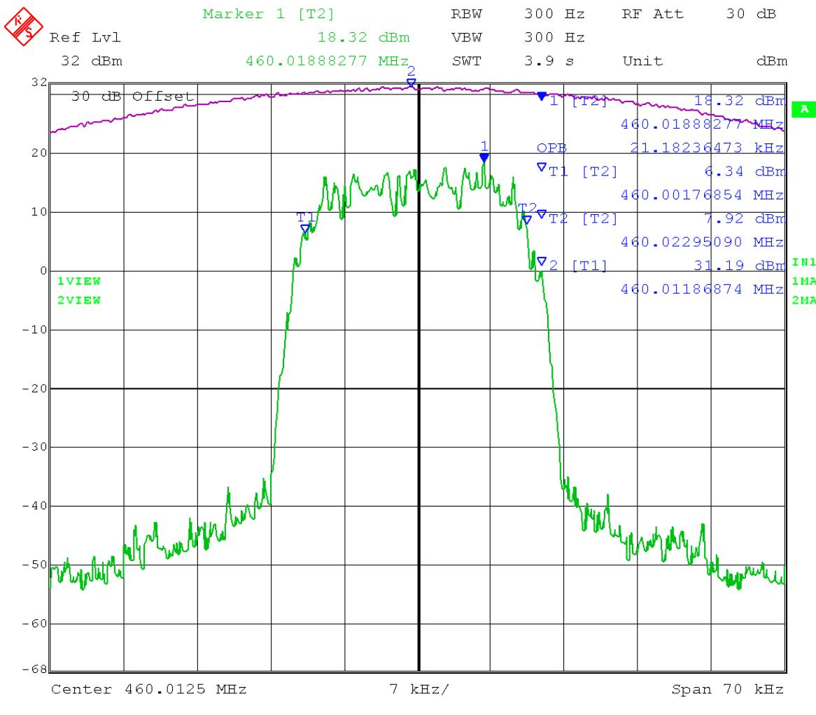
99% OCCUPIED BANDWIDTH = 21.18 kHz (460.01 MHz)
