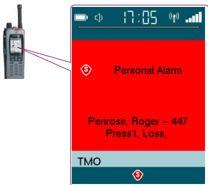
Display after an alarm is triggered (here: pressure alarm 1)
