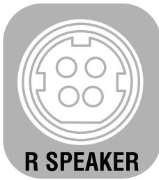
These ports (present on both speakers) allows you to connect the active speaker (Left port) with the passive speaker (Right one). These are 4 pins connectors: in this way is it possible to carry the powered signal both for the HF driver and the LF driver.
