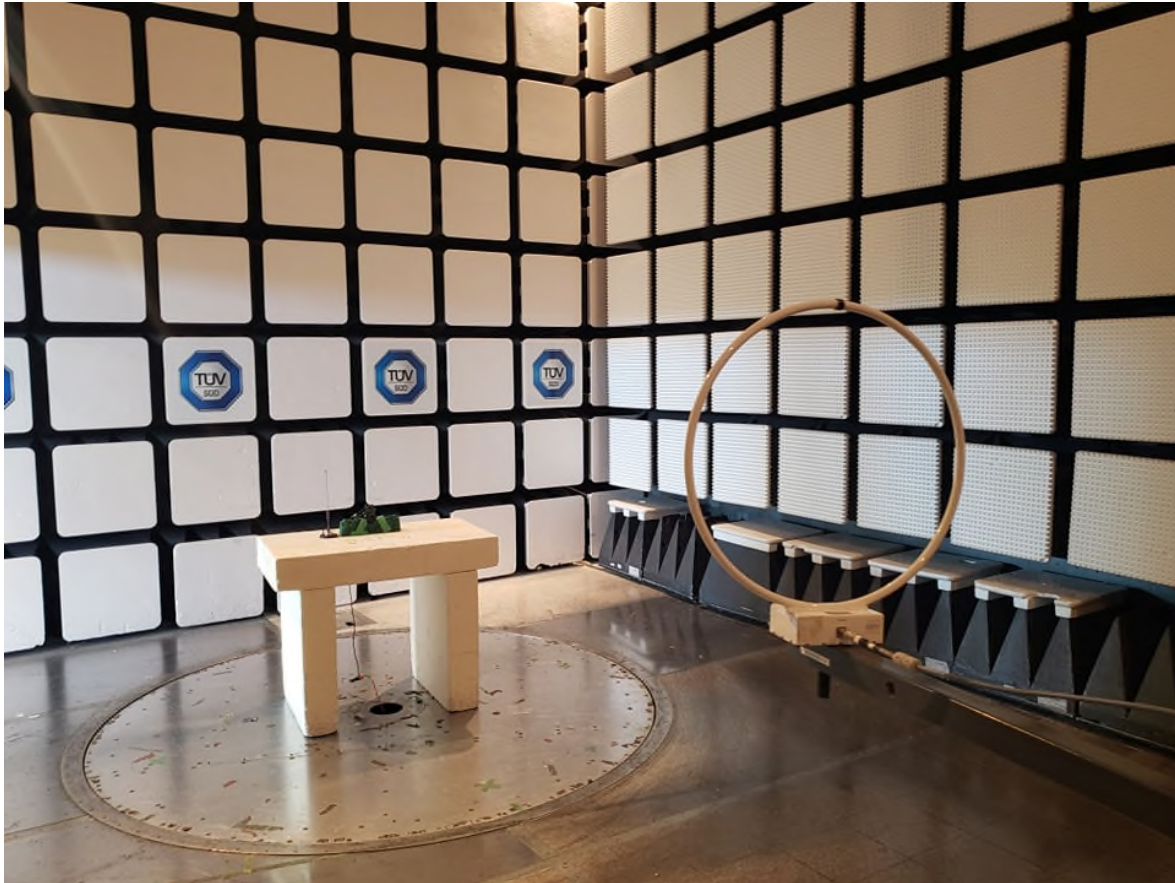
Figure 2 – Radiated Emissions Setup 9kHz – 30MHz
