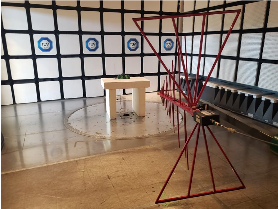
Figure 3 – Radiated Emissions Setup 30MHz – 1GHz
