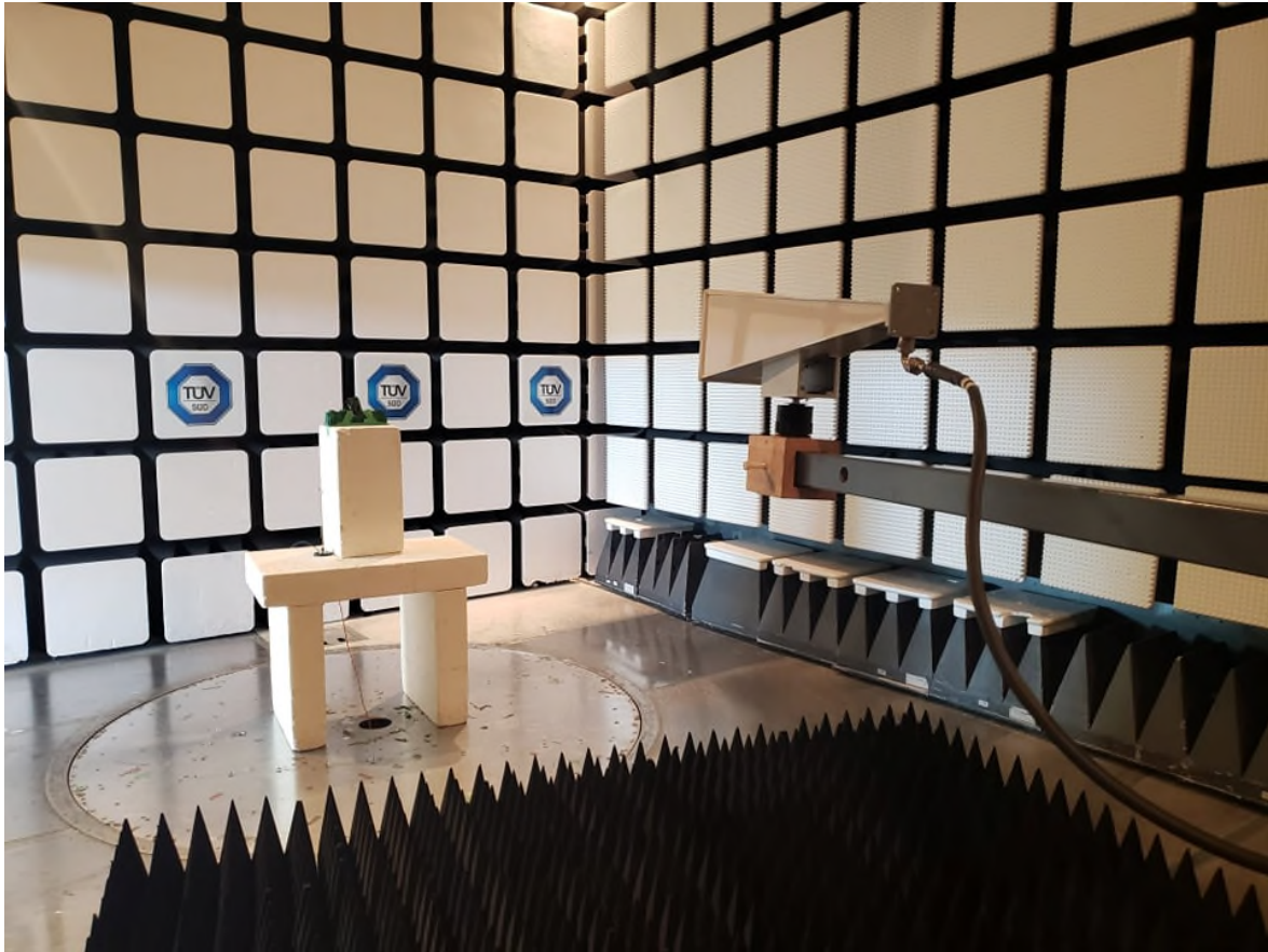
Figure 5 – Radiated Emissions Setup 6GHz – 10GHz
