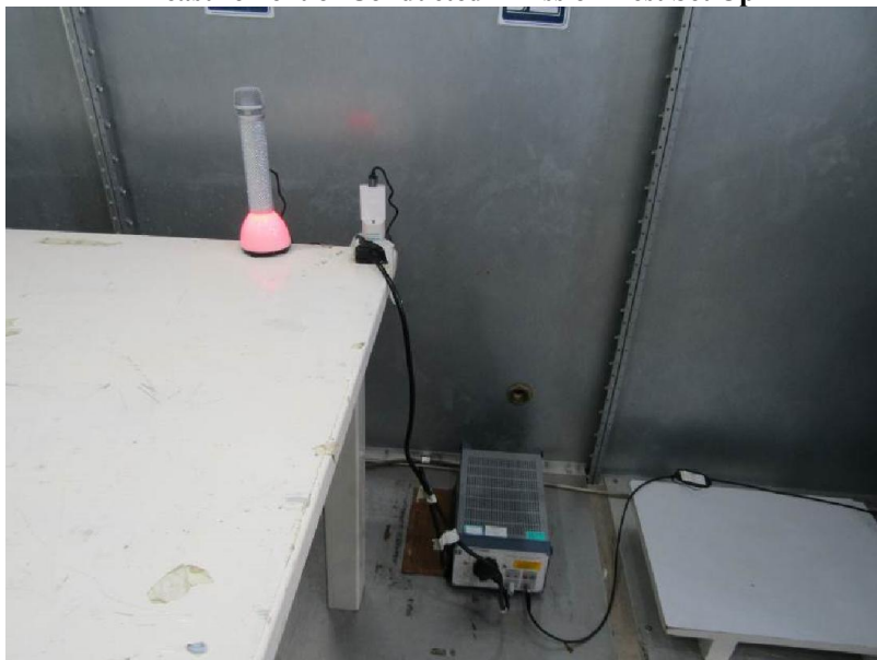
Measurement of Conducted Emission Test Set Up
