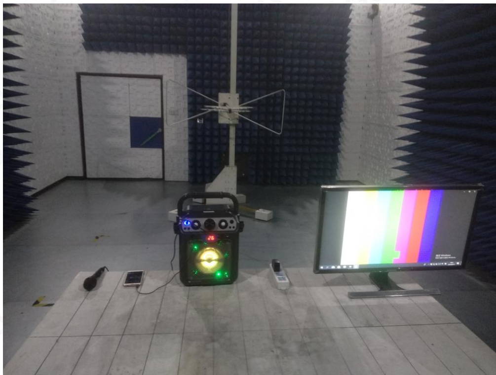
RADIATED EMISSION TEST SETUP ABOVE 1GHZ
